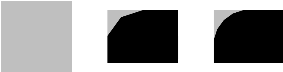
FIGURE 9.10. On the left, we show a square in gray. In the middle, we zoom in on a corner of the square. Overlaid on the corner in black, we show the opening of the square by a regular polygon with 10 sides. On the right, we show the opening of the square by a regular polygon with 20 sides. When we double the number of sides in the polygon, the number of edges at a corner of the square also doubles. While the number of sides in the square remains constant, the number of sides in the opening is linear in the number of sides in the polygon used for opening.
