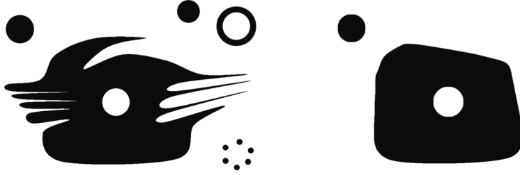
FIGURE 4.1. (Left) The input binary image consists of 1102 x 832 pixels. (Right) The tightening of the input with a radius of 40 pixels.
