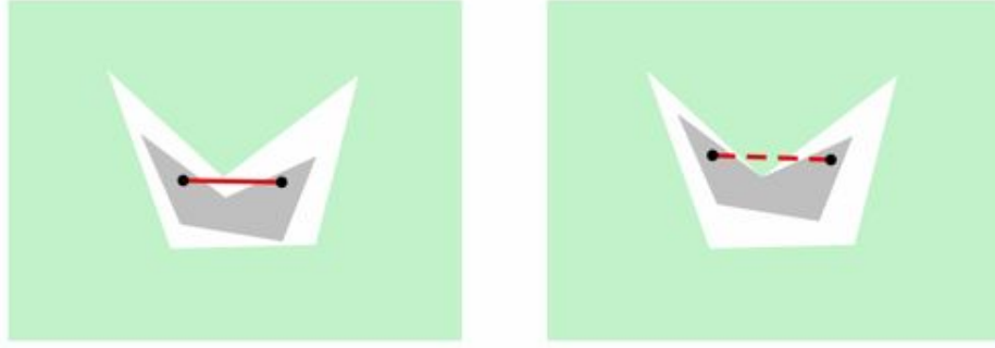
FIGURE 6.9. The set S shown in gray on the left is not convex relative to the green set G because the red line segment connecting the two black points is not contained in S despite the fact that it is disjoint from G . The set shown in gray on the right, by contrast, is convex relative to G .
