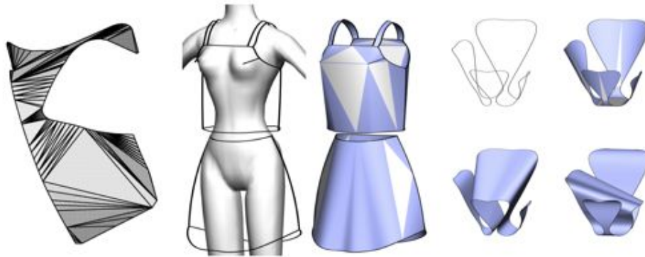
FIGURE 10.7. On the left, we show a triangulation of a boundary curve [30] that estimates the geometry assumed by a sheet of metal pressed by a machine. The center image [57] illustrates garment design by interpolating seams with developable patches. The right images [57] show how multiple patches can interpolate the same boundary curve, providing us with motivation to determine which patch is “best.”
